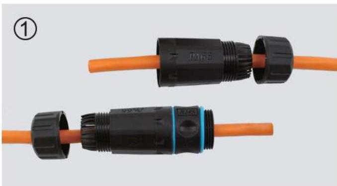
1. Attach the central tube to one long tube. Pass one cable through end cover & long tube and the other cable through end cover & long tube & central tube.
