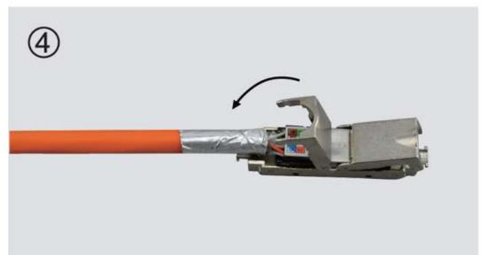
4. Place wiring cap assembly into the cable joiner. Close the cover and repeat for the second cable.
