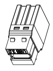
Connector Contact: 15U" Gold Plating Contact Resistance:  $30m\Omega$  (max) Insulation Resistance:  $10M\Omega$  (min) Voltage Rating: 30 VDC (rms) Insertion Force: 35N (max) Extraction Force: 10N (min)
