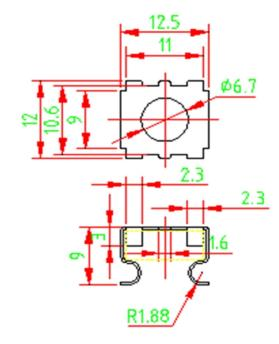
Code: CageNut4PT CageNut50PT M6 M6 screw nut (thickness 4.5mm) 4.75 Materials:
