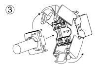
Insert the loaded termination cap into the socket, ensuring the arrows face the same direction. Evenly press the 'wings' together
