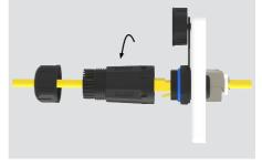
2. Pass the patch cord through the end cover and the long tube. Then insert the connector. Tighten the long tube.
