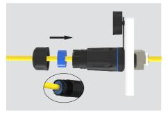
Lock the waterproof plug on the cable, then put it into the end of the long tube.
