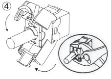
Ensure the socket is completely closed, pliers can be used. Ensure continuity of shielding
