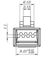
SPECIFICATIONS 1.ELECTRICAL: UL APPLICATIONS: 250 VOLTS AC MAX. AT 2 AMPS. DIELECTRIC WITHSTANDING VOLTAGE : 1000 VOLTS AC. 60 SEC. INSULATION RESISTANCE: 500 MΩ. CONTACT RESISTANCE: 20mQ MAX. OPERATING AMBIENT TEMPERATURE: -40°C ~ 70°C. 2.MECHANICAL: STRAIN RELIFE: 20POUND MIN. DURABILITY: 1200 MATING CYCLES.
