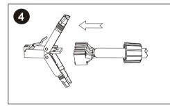
Push cable and core carrier onto the PCB.
