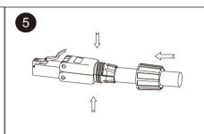
Firmly close and secure by screwing on the end cover.
